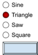
Figure 3 Example of a Device using a button to cycle through the options
